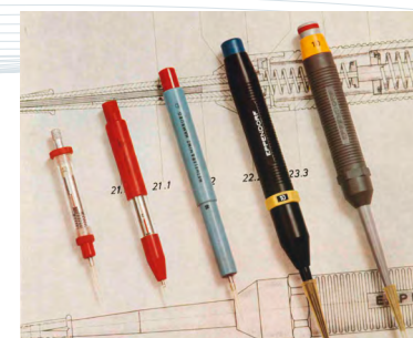
Developmental stages of the first Eppendorf micropipettes in the 1960s.
