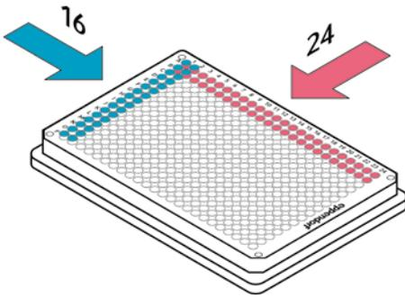
Fig. 2: Pipette entire rows (24 channels) or columns (16 channels) in a single step
