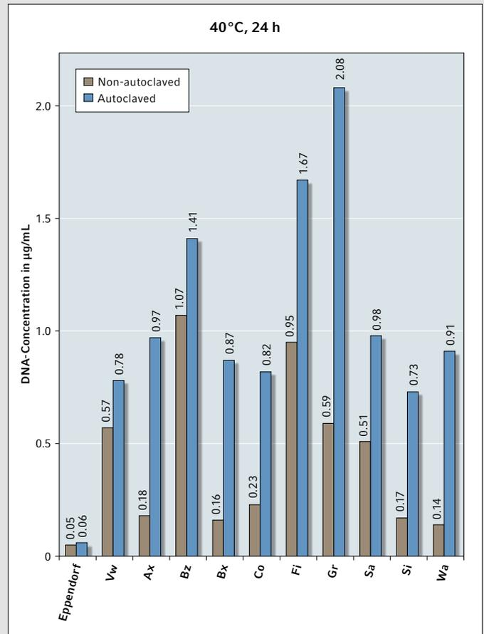
**Fig. 1:** False DNA concentration (µg/mL) based on UV-absorbing leachables, which had been released from micro test tubes into ultra-pure water samples after incubation at 40°C, 24 h. Mean values of 24 pooled samples from non-autoclaved (brown bars) and autoclaved (blue bars) tubes are shown.
