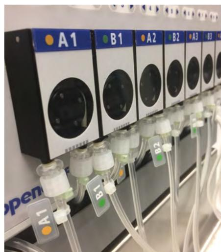
Fig. 2: Feed line with new label, consisting of cable tie, identification plate, and adhesive label
