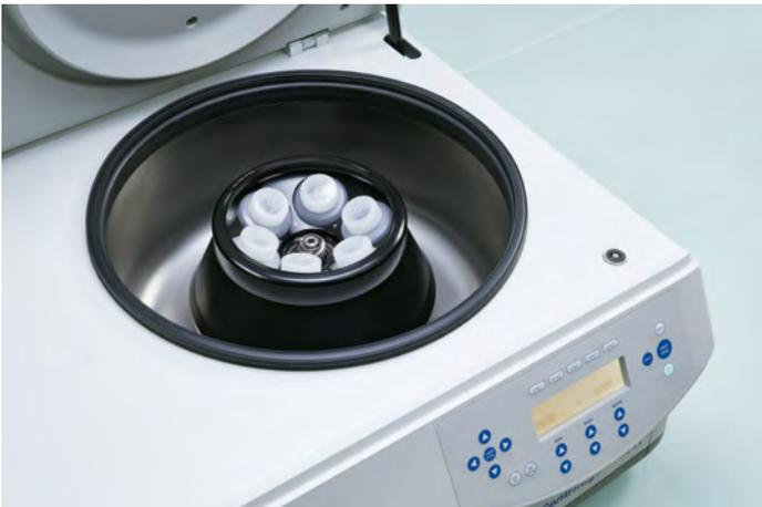
High-capacity fixed-angle rotor for a broad range of applications with max. speed of 15,054 x g (10,100 rpm)
