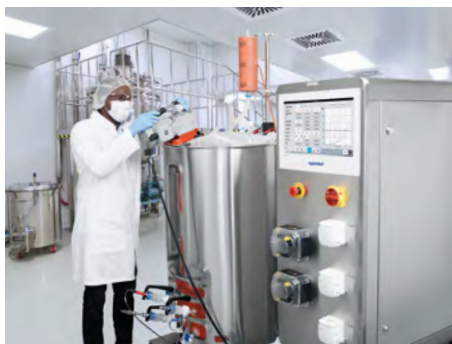
The BioFlo 720 bioprocess control station is compatible with the Thermo Scientific HyPerforma 5:1 single-use bioreactors with working volumes of 50 L and more
