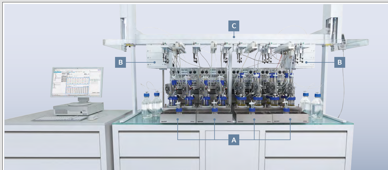
Fig. 1: DASbox Mini Bioreactor System equipped with the Bioprocess Autosampler. A: DASbox Mini Bioreactor System. B: Cooling stack. The cooling stack has three drawers. The temperature of the cooling stack can be regulated from 4°C to 40°C. C: Robotic arm equipped with liquid tools
