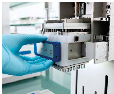
Quick and easy: exchange of the dispensing head
