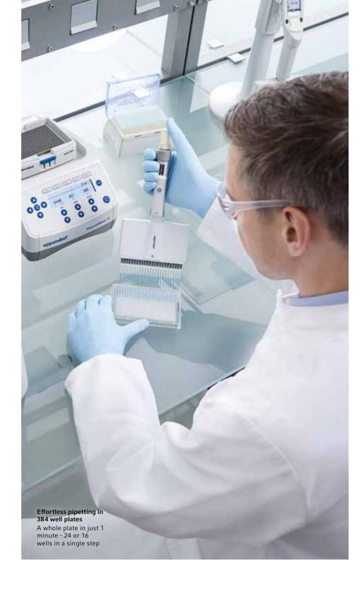
t is understandable if scientists prefer to avoid this replacement, as manual work involving the 384-well format is no picnic, and automation is not always a feasible solution. Who is not familiar with the cumbersome "staggered pipetting" using 8 and 12 channel pipettes? This common technique requires extreme concentration; it is time-consuming, and it carries a risk of error – particularly under stressful conditions.
