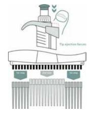
SOFTeject reduces ejection forces by 50%
