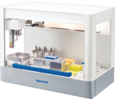
The first product to be launched in the new design was the epMotion at the beginning of 2023. The pipetting robot not only boasts a new, modern, high-quality and functional design, it has also been enhanced with new features, including various software functions and a large waste drawer that is concealed behind the silver protective belt. In making this upgrade, Eppendorf has responded to specific customer requests.
